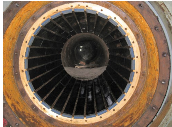
ROMOR® I Naval Bronze Dovetail Housing System.
